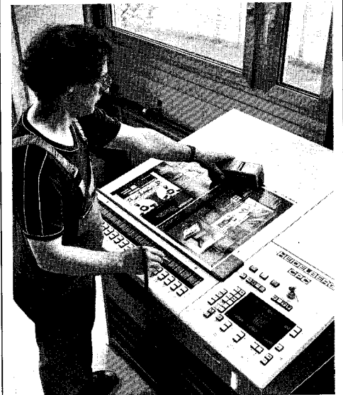
CPC station for controlling and storing important machine parameters such as inkage, ink zones or register (register tolerance of the individual colors).
